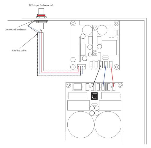
When using RCA inputs do NOT connect chassis to safety earth to avoid ground loops. Amplifier must be build according to double insulation safety standards.
